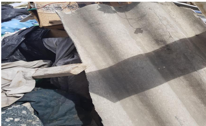
Photo 3.12 Asbestos waste, once used for roofing, is not treated with the needed security measures and ends up mixed with other waste in the environment. Photo: Nagon, 2019
